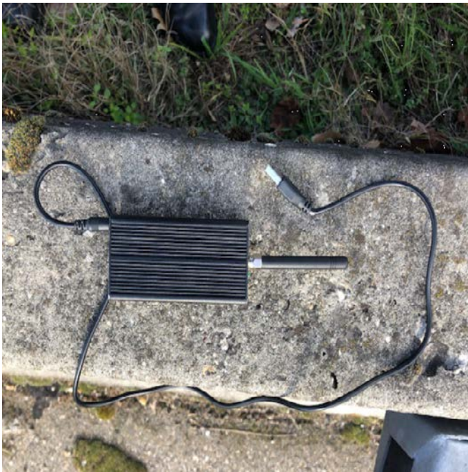
Figure 2: A GPS spoofing device seized during an intervention by the ANFR. Source: ©ANFR
