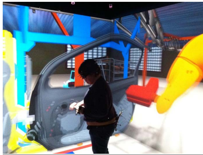
Figure 6: Virtual reality for simulating a workstation with a collaborative robot: the operative is interacting via an immersive system (WEISTROFFER 2014).
