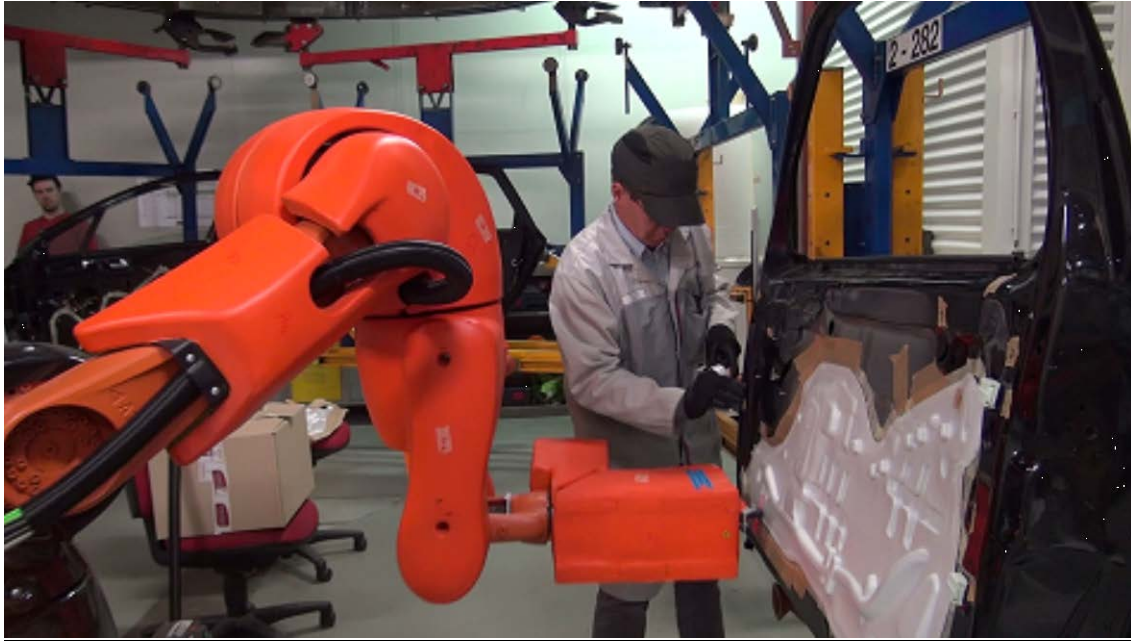
Figure 1: Assembling a door on a vehicle in coexistence with a robot (WEISTROFFER 2014).
