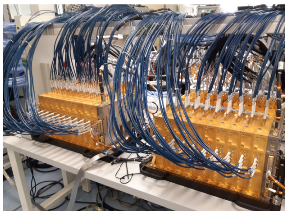
Figure 8 : Digital Transparent Processor NG (© Thales Alenia Space).
