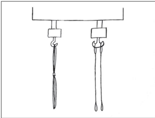
Figure 6: Traveling crane prepared for hoisting (drawing made during fieldwork).
