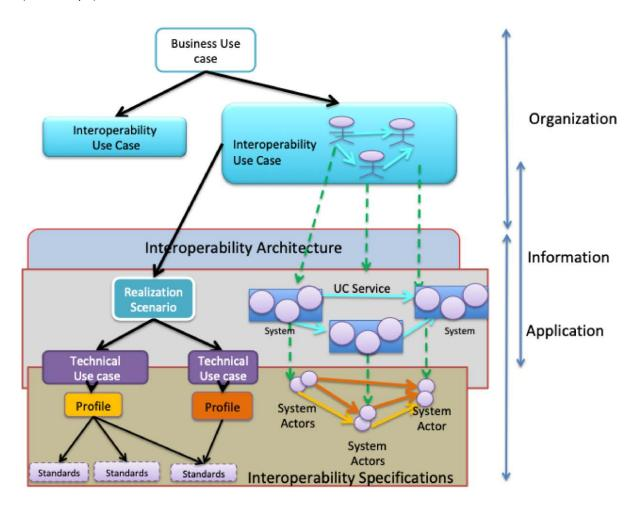
Whereas standards are general enough to respond to all uses, INTEGRATION PROFILES are specifications for use case implementation (Figure 2). Such a profile assembles a set of standards that have to work together to handle use cases (*e.g.*, data series or message formats). Two major consortiums are developing integration profiles in the health field: Integrating the Healthcare Entreprise (IHE) and PCHA/Continua Alliance for connected health devices.
