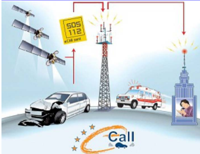
Figure 3: eCall, a system for emergency calls.
