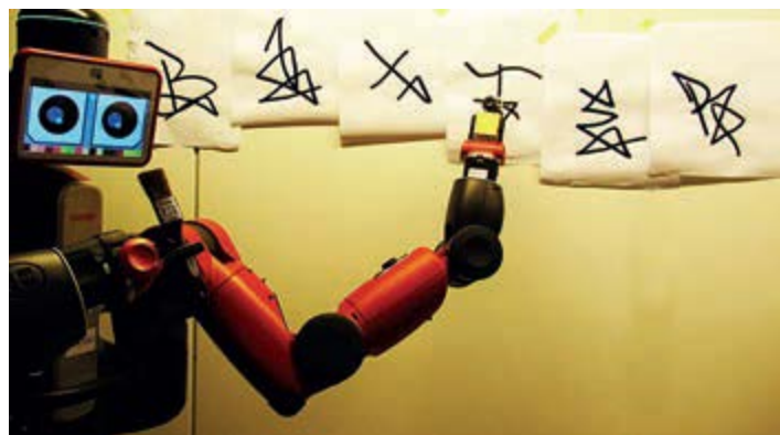
Figure 8: Baxter, a nonrigid humanoid robot designed by Rethink Robotics, learned to write its own tags of a quality close to what a human being can do (BERIO et al. 2016).
