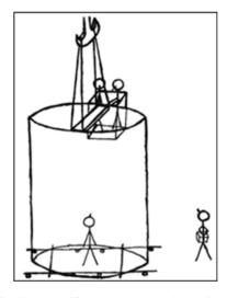
Figure 5: Positioning a lifting beam on a cylinder (drawing made during fieldwork).
