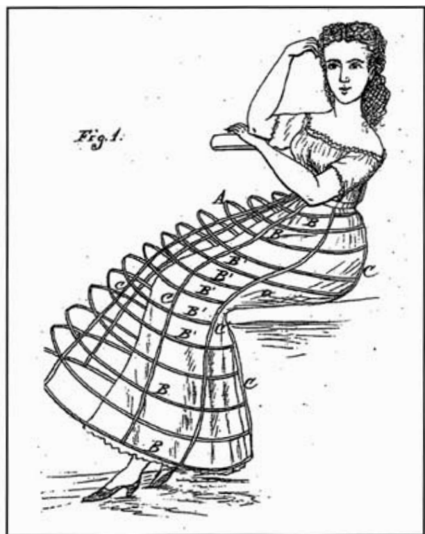
Figure 2 : Patent for crinoline that makes it easy to sit down.
