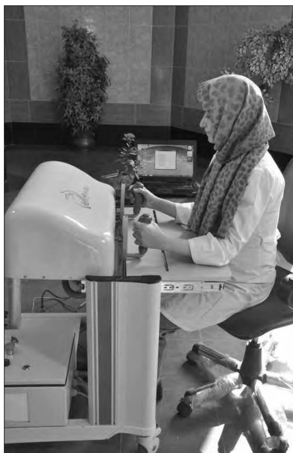
Figure 5: Wrist-RoboHab, the robotic upper limb rehabilitation system developed at RCSTIM.
