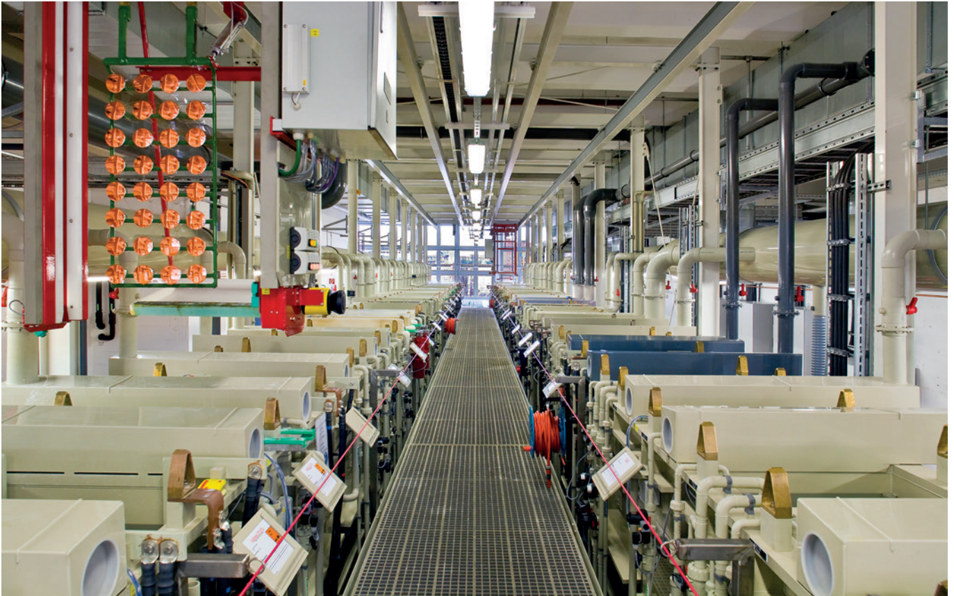
General Metal Finishing: Plating on Plastics pilot line installed in Berlin Tech Center for development, customer samplings and qualification runs for automotive industry.
